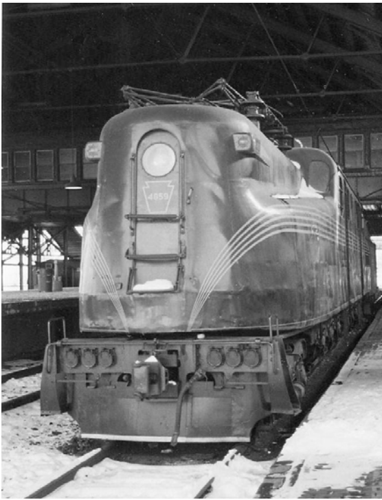
A fleet of 139 GG1 electric locomotives was produced for the PRR utilizing a modern, streamlined design in 1937. One of the fleet inaugurated the electrified service on the Philadelphia-Harrisburg: GG1 Locomotive No. 4859 (above), which has been preserved on Track 5 at the Harrisburg Transportation Center and is listed on the National Register of Historic Places, pulled the first electrically powered train over the route on January 15, 1938.
